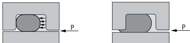
The reference values given in the table for gap dimensions for standard elastomer are maximum values based on central alignment of the components. The permissible values for the sealing gap are dependent on pressure, material hardness and diameter. All specifications are based on experience and should only be regarded as guideline values.
