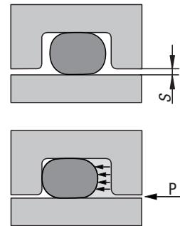
An O-ring is used primarily for static seals. They have only limited use as dynamic seals in hydraulics and pneumatics (dependent on the pressure, speed and temperature). Due to frictional resistance, the compression for dynamic use should always be calculated less than for static applications. Sufficient lubrication should always be ensured during dynamic applications.
