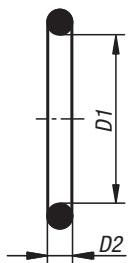
An O-ring is a sealing element used to reliably seal against fluids and gases. The seal effect is created during installation by axial or radial compression of the cross-section. During operation, the pressure of the medium intensifies the deformation of the O-ring and enhances the sealing function.
